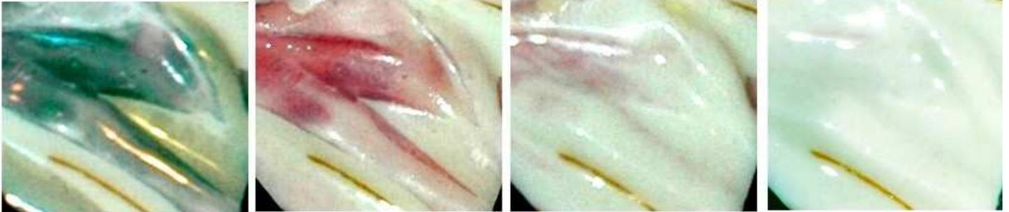
This item, which was left immersed in undiluted lemon juice, refreshed and topped up as required, shows marked changes in the colour and intensity of the lustre with time:
