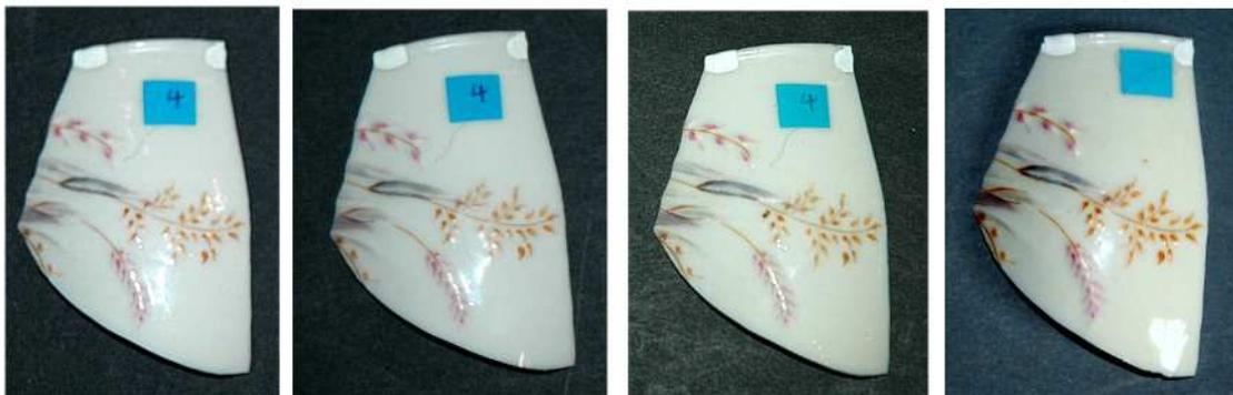
**Item 4:** Shard from a cup, exposed to sunlight through glass, facing upwards, on a South-facing windowsill.
