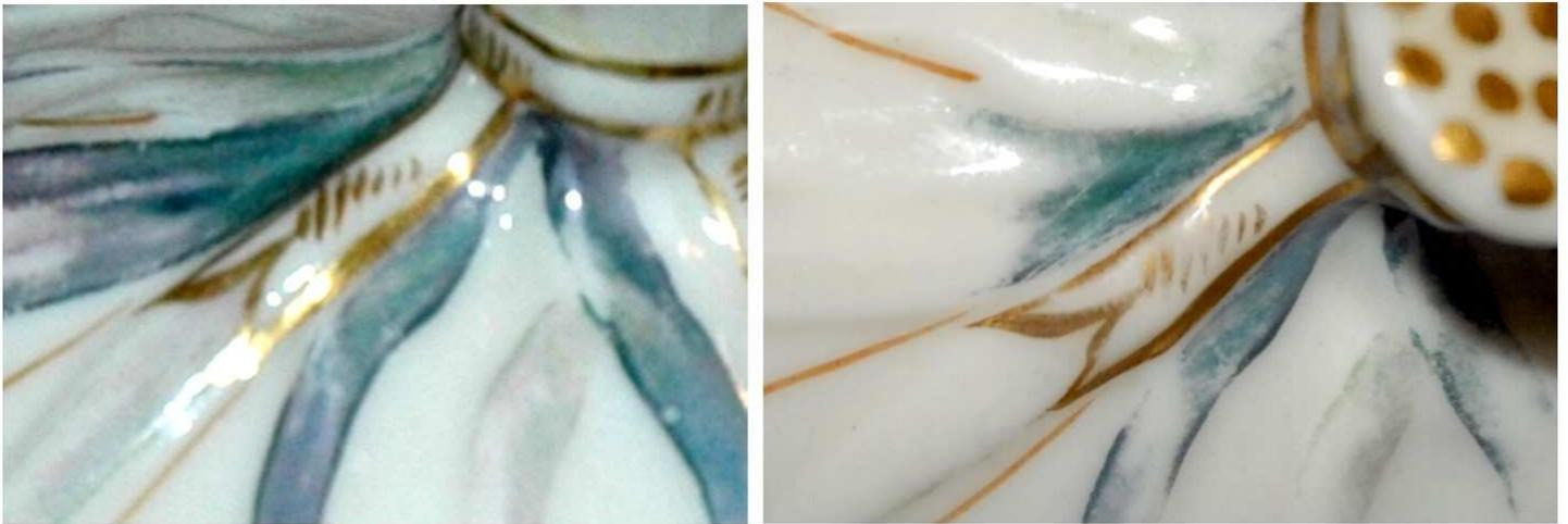
This shows that the repeated scrubbing of the sugar bowl with a scouring sponge has caused wear to the lustre decoration and *also to the gilding*. This wear is caused by mechanical rubbing rather than any effect of the water or washing-up liquid and is only to be expected given the extreme nature of the treatment. The loss to the decoration is on the more raised and accessible parts of the item.
