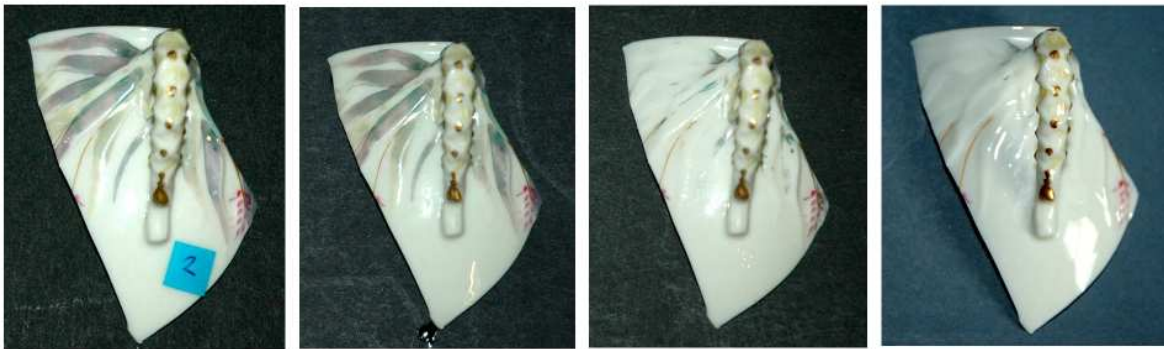
Item 2: Part of a cup with handle attached - immersed in Chlorine Bleach.
